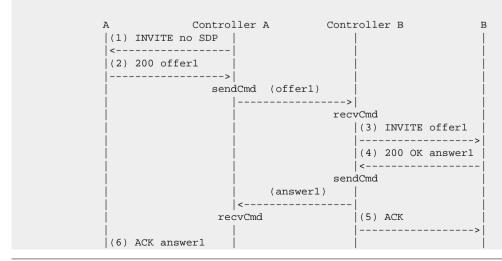
As you can see, we need to pass information between both sides of the controller. SDP "offer1" is provided by A in message (2) and needs to be sent to B side in message (3). This mechanism is implemented in the scenarios through the <sendCmd>command. This:
