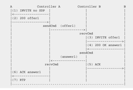
As you can see, we need to pass information between both sides of the controller. SDP "offer1" is provided by A in message (2) and needs to be sent to B side in message (3). This mechanism is implemented in the scenarios through the <sendCmd> command. This:
