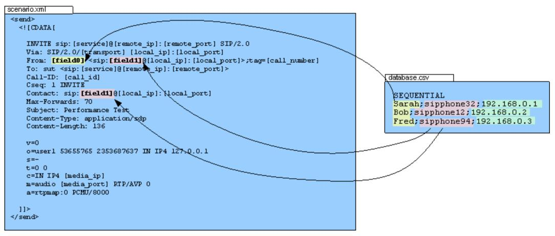
This mode is generally used for emulating user agents, using on IP address per user agent and calling a SIP server.
